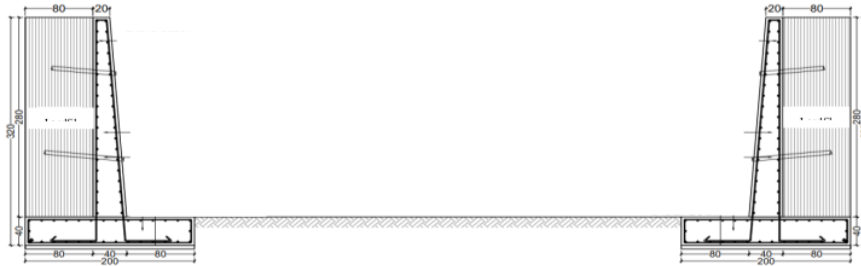
Figure 4. Alternative 2 (Concrete Sheet pile)
