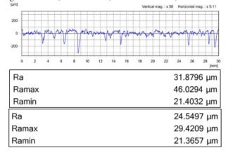
From the surface profile results, it can be observed that the surface of the concrete produced by the conventional wood method has an uneven contour with several concave holes indicated by the depressions in the profile readings. From the observations, these holes are caused by air bubbles trapped in the concrete mix during wet conditions. Meanwhile, for the overall surface roughness, the average roughness (Ra) from both observations is found to be
