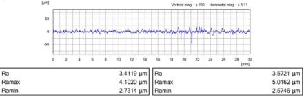
From the results of surface profile, it can be observed that the surface is very smooth but still has contours. Only depressions due to the pattern of the PERI DUO polymer formwork surface were found in the concrete surface samples during the observation. Meanwhile, for the overall surface roughness, the average roughness (Ra) from both observations is  $3.492 \mu m$ .
