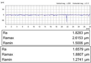
From the surface profile results, it can be observed that the surface contour is very smooth, with no observed concave holes in the concrete surface samples. Meanwhile, for the overall surface roughness, the average roughness (Ra) from both observations is found to be  $1.7431 \, \mu m$ .
