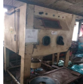
Figure 26: Sand blast machine
