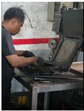
Placement of the rubber sheet on the mould
