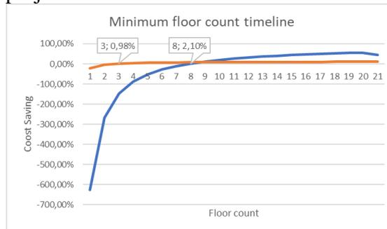
The minimum number of floors for this alternative use can also be seen from the table where the minimum floor count The film plywood will begin to achieve savings on a minimum of 3 floors, while for DUO polymer, savings will be realized for usage on a minimum of 8 floors.
