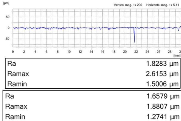
From the surface profile results, it can be observed that the surface contour is very smooth, with no observed concave holes in the concrete surface samples. Meanwhile, for the overall surface roughness, the average roughness (Ra) from both observations is found to be **1.7431  $\mu\text{m}$** .
