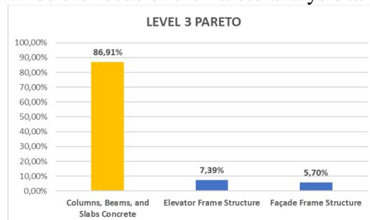
In the Pareto analysis at level 3, the highest percentage is obtained for the concrete work of columns, beams, and slabs, amounting to 86.91%. The Pareto analysis is then continued at the next level, which is level 4.
