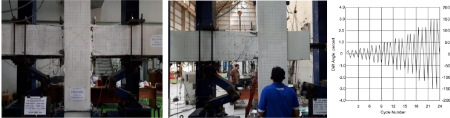
Fig. 19 – Beam column joint test
