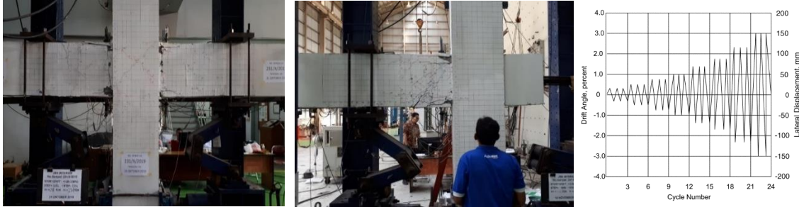
Fig. 19 – Beam column joint test
