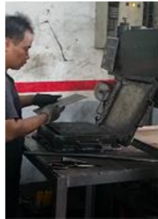
Placement of the steel plate on the mould
