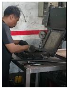
Placement of the rubber sheet on the mould
