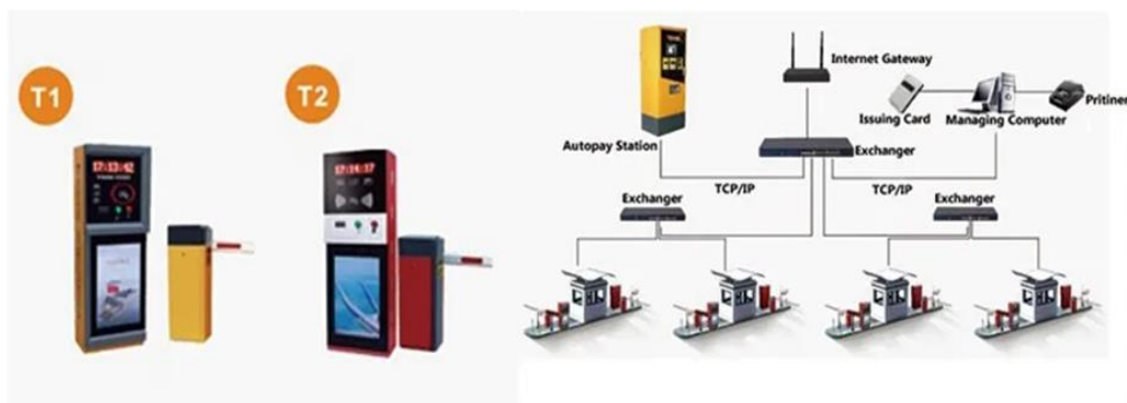
Figure 4. Smart Parking Management System
