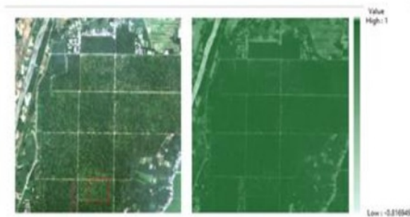
Fig 3:- Comparison of original colow imagery composite (a) and NDVI value in some part of research location (b)
