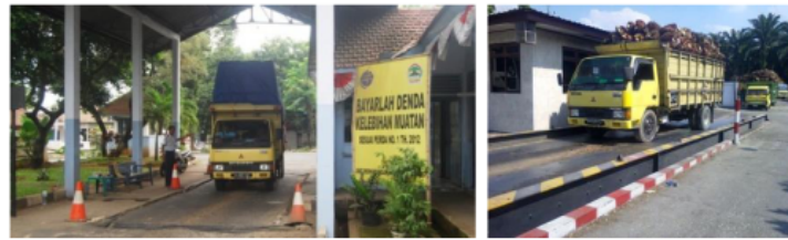
Fig. 4. Control vehicle load by weighbridge
