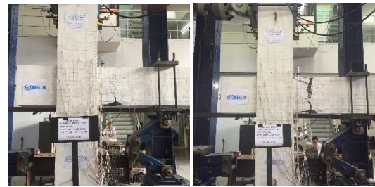
(a) Drift at 1.75% (b) Drift at 3.5%
