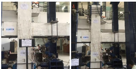
(a) Drift at 1% (b) Drift Until 1.4%
