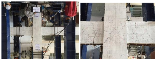
(a) Drift at 1% (b) Drift Until 2.2%+
