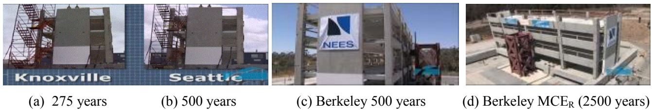
Fig.3 – Testing of high performance earthquake resistant structure with shaking table equipment
