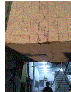
(a) service limited \Delta = 0,35\% , equal V (b) gap in upper side \Delta = 1.75\% (c) gap in bottom side \Delta = 1.75\%
