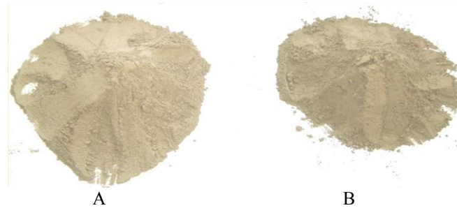
Figure 1 (A) Organic cement made from organic garbage. (B) Portland cement
