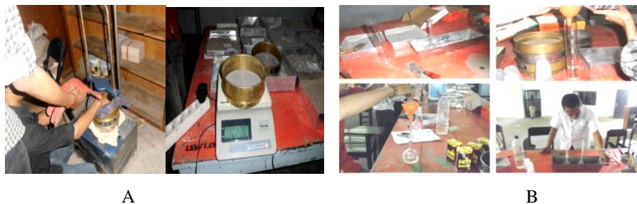
Figure 2 (A) Organic cement examination process. (B) Organic cement specific gravity examination.
