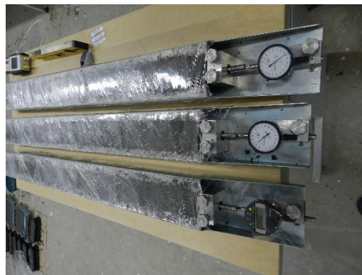
Figure 3 Autogenous Shrinkage instruments
