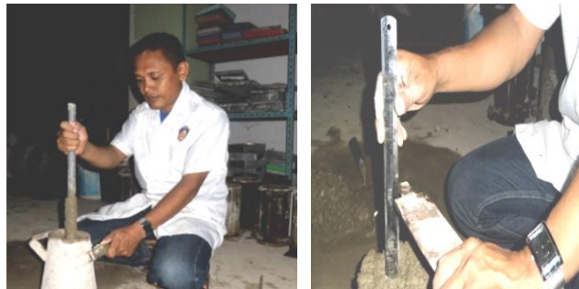
Figure 4 Slump test of fresh concrete
