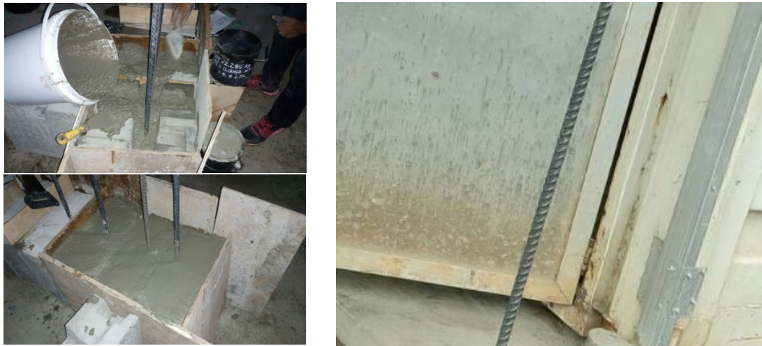
Figure 6 Preparation and final form of specimens for pull-out test on dowel activator
