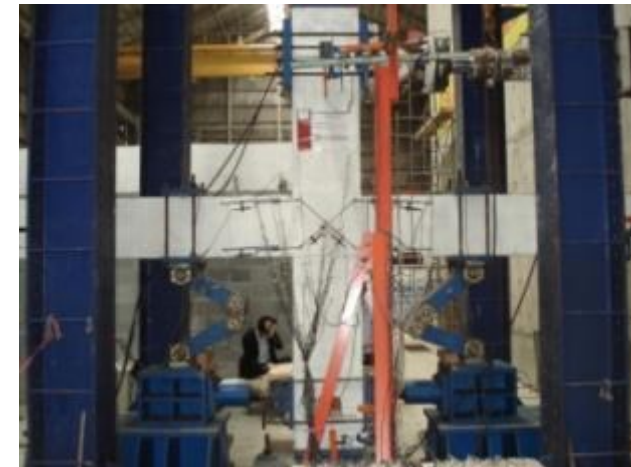
Earthquake test of interior precast joint
