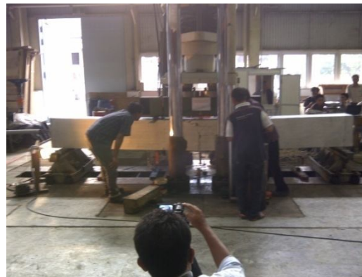
1.4% - Tension gap widening at Dissipater and compression failure
