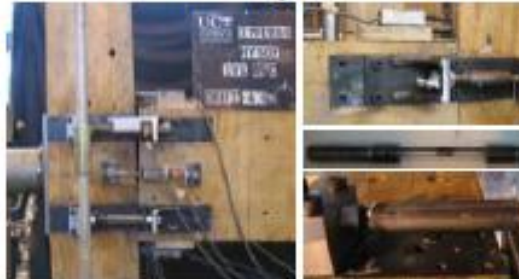
EXTERNAL DISSIPATERS: mild steel rods with epoxied encased steel tubes
