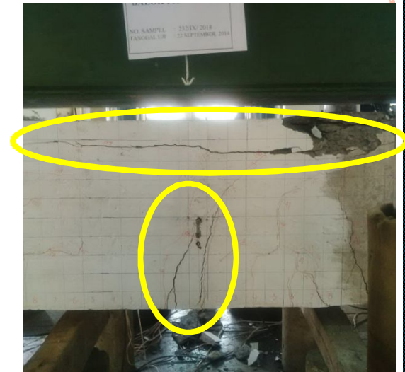
1.7% - 2 crack line in dissipater dan
