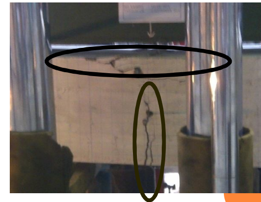
1.4% - Tension gap widening at Dissipater and compression failure
