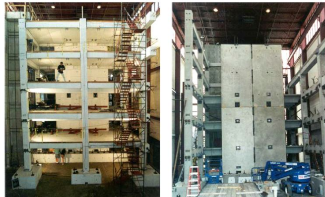
Figure 25 Five-Storey PRESSSS Building tested at University of California, San Diego [13]
