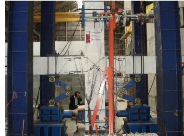
Earthquake test of interior precast joint
