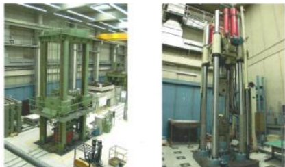
LOS UBP 15000 kN pressure testing machine (height of testing room approx. 7 m)
