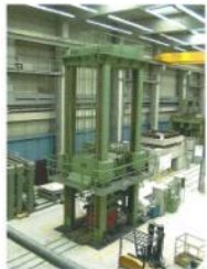
LOS UBP 15000 kN pressure testing machine (height of testing room approx. 7 m)
