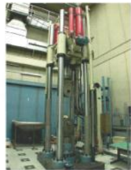
MTS 2500 kN testing machine for tension and pressure up to a load velocity of 1800 mm/s
