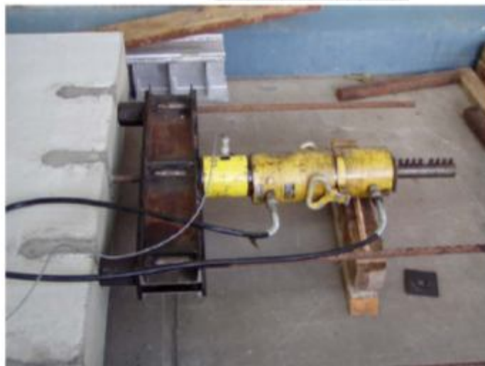
Figure 3-2: Pull-out test setup for Test 1
