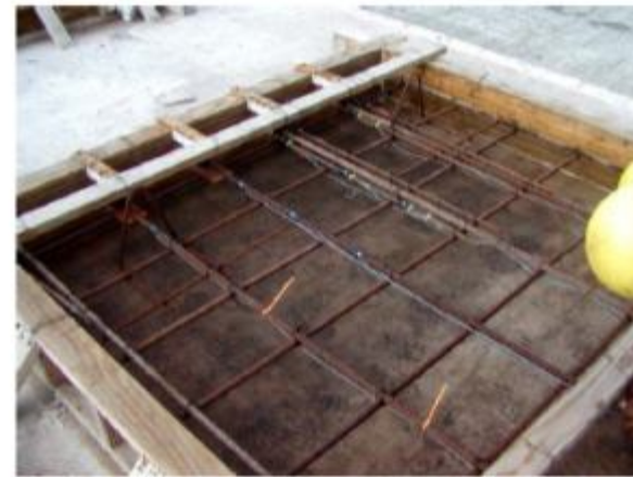
Figure 2-8: Kwik Joint pull-out test panel prior to concrete placement
