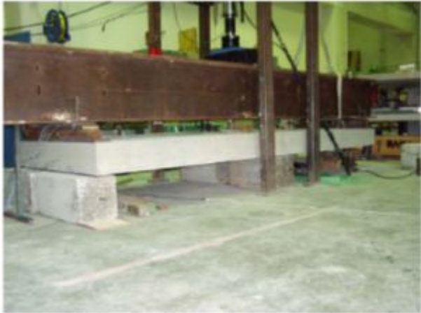
Figure 3-5: Flexure test in load frame
