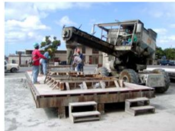
Figure 2-8: Kwik Joint pull-out test panel prior to concrete placement
