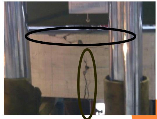
1.4% - Tension gap widening at Dissipater and compression failure
