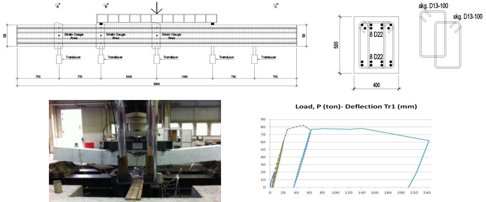
Table 1. Test analysis of reinforce concrete beam specimen ( $M_o = 615 \text{ kN m}$ ,  $P_o = 410 \text{ kN}$ )
