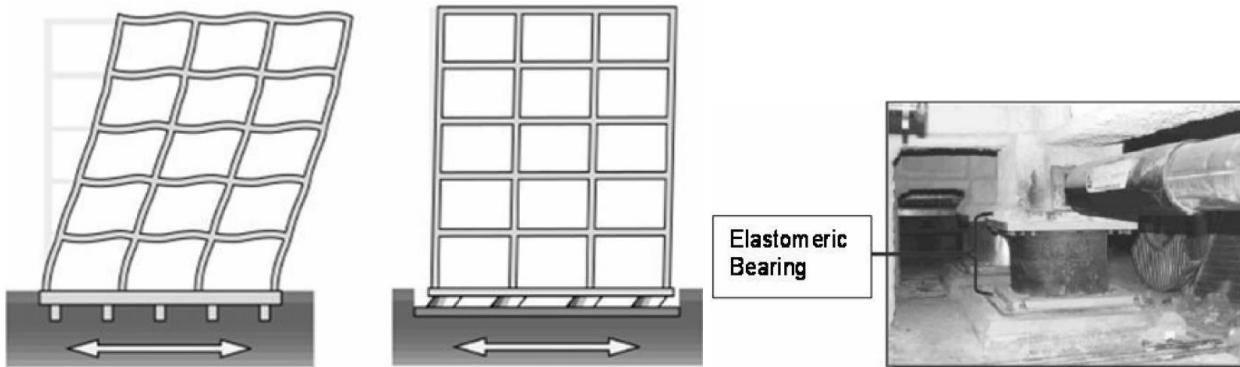
Figure 20 Base insulation concept [7]
