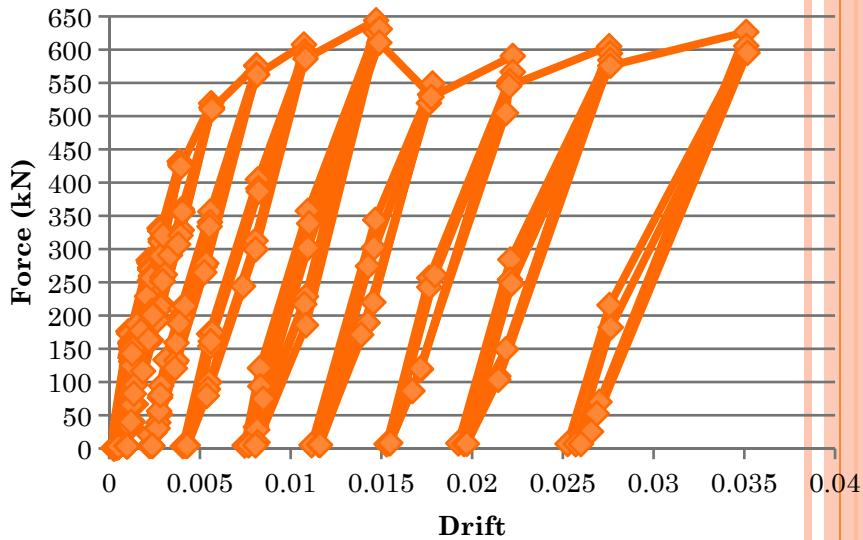
3.5% - speciment still sustain, game between compression confined concrete at dissipater and tension of steel
