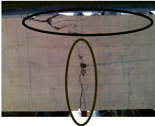
1% - Tension Gap at Dissipater and compression failure
