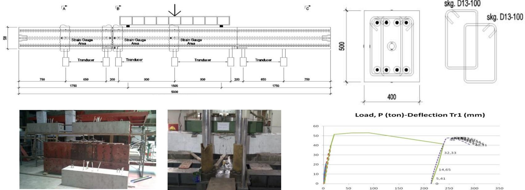
Table 4. Test analysis of segmental hybrid beam specimen ( $M_o = 615 \text{ kN m}$ ,  $P_o = 351 \text{ kN}$ )
