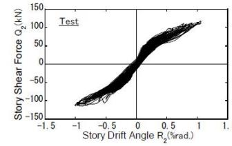
Test Shaking Table Sistem PRESSS (Maruta,Jinhua,2012)
