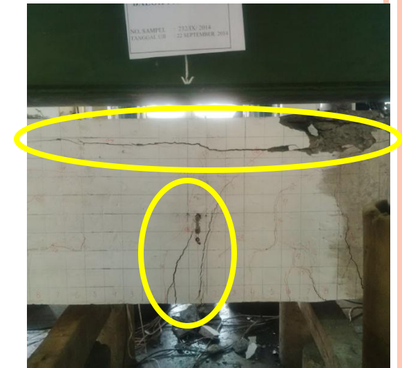
1.7% - 2 crack line in dissipater dan
