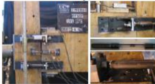
(a) Internal and external dissipaters and construction details.
