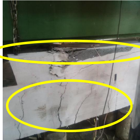
2.2% several tension crack occur – As enter strain hardening phase
