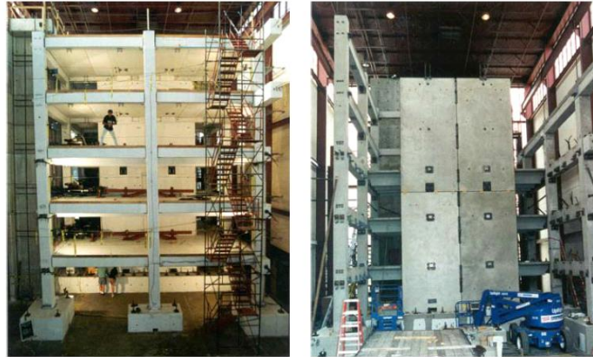
Figure 25 Five-Storey PRESS Building tested at University of California, San Diego [13]
