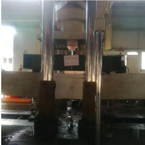
2.2% several tension crack occur – As enter strain hardening phase
