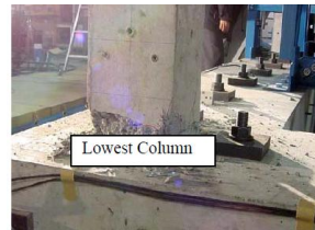
Test Shaking Table Sistem PRESSS (Maruta,Jinhua,2012)
