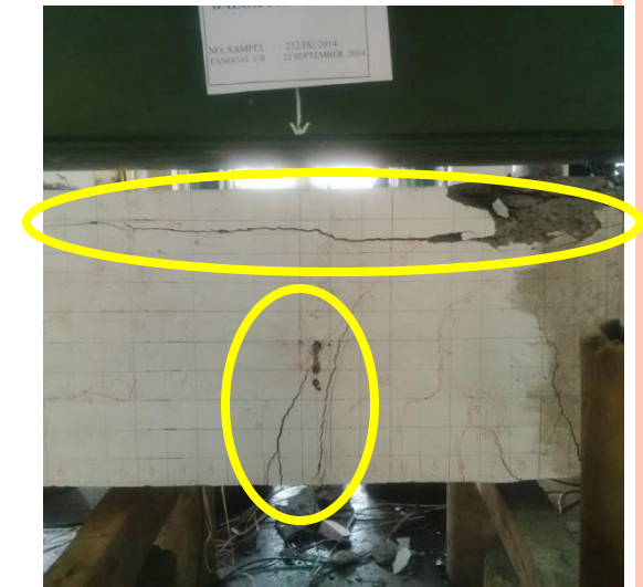
1.7% - 2 crack line in dissipater dan
