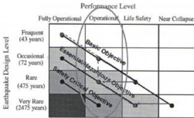
Figure 3.1- Seismic Performance Design Objective Matrix (after SEAOC Vision 2000, 1995) and proposed modification of Basic Objective towards damage control (dashed blue line)
