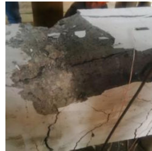
3.5% - speciment still sustain, more and more tension crack and
