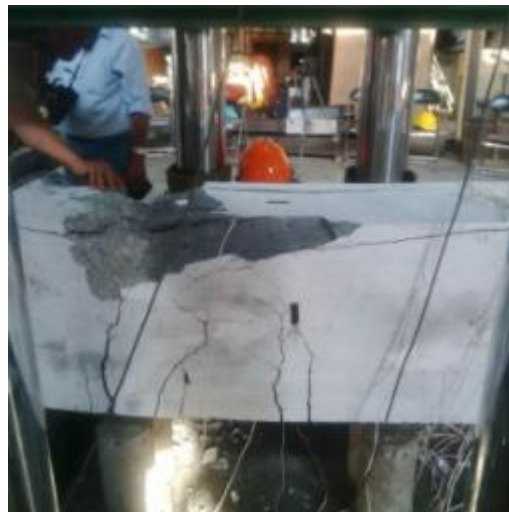
3.5% - speciment still sustain, more and more tension crack and
