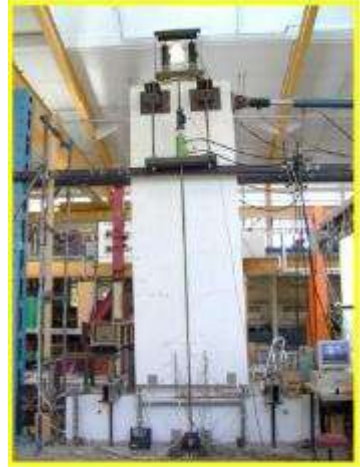
Overall View at 3% Roof Drift Ratio
