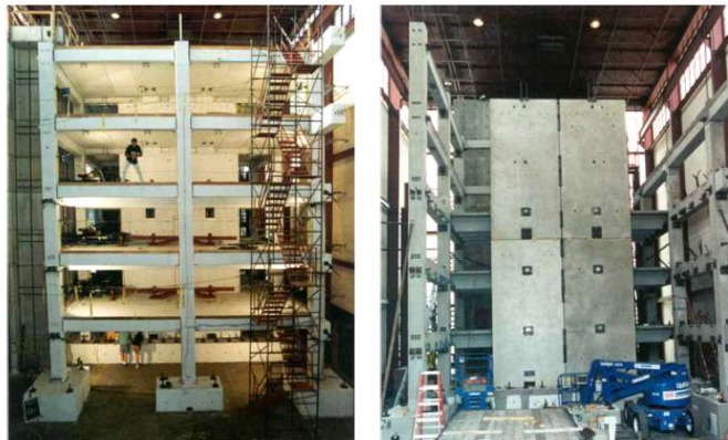
Figure 25 Five-Storey PRESSS Building tested at University of California, San Diego [13]
