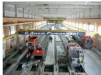
Echo Precast Engineering equipped the Domodedovo works of the SU-155 construction group with a production plant for prestressed hollow core slabs.
