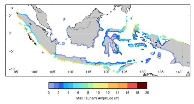
Fig. 4 – Tsunami hazard map of máximum tsunami amplitude (m) at Coastal line with return period of 500 years [7]
