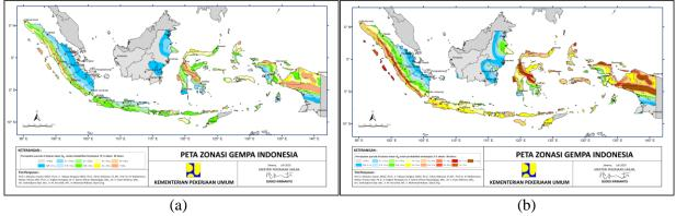
Fig. 3 – Peak Ground Acceleration (PGA) seismic hazard map at bedrock (S<sub>B</sub>) for (a) 10% probability of exceedance in 50 years, (b) 2% probability of exceedance in 50 years
