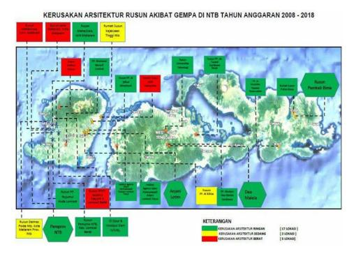
Fig. 8 – Map of architectural damage on housing flats in Lombok, Sumbawa, Bima and Mataram due to earthquake
